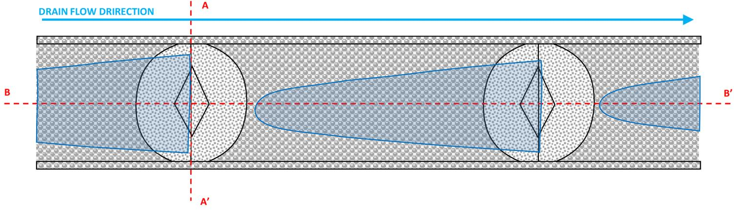
**Constructed Drain and Check Dams – Section A-A'**
