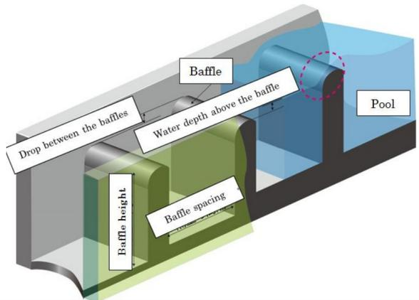
**Conceptual graphic of weir pool and the use of baffles**
